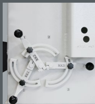
Manual adjustment of the 3 flaps
