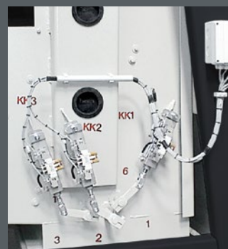
Electro-pneumatic adjustment of the 3 flaps
